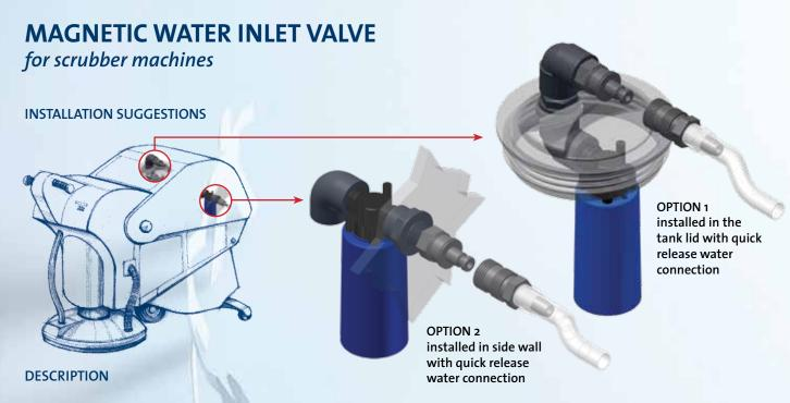
The Abertax Technologies Magnetic Water Inlet Valve features a float with an embedded magnet that will operate a diaphragm type valve. The rising water level lifts the float. The magnet inside the float then moves a stainless steel pilot plunger which closes the valve.
