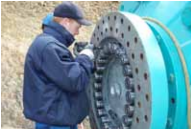
Flange coupling of the gear box on a wind turbine. An Expansion bolt with integrated Superbolt technology is used to transmit the enormous torque. The solution is also compact and does not add a lot of weight, which was a requirement.
